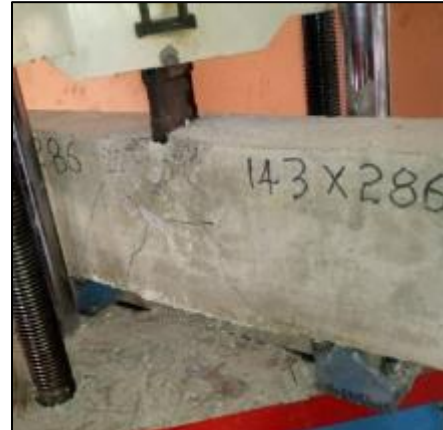
Figure 9 143 x 286 mm Deep Beam after loading to failure
