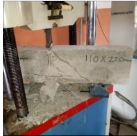
Figure 5 110 x 220 mm Deep Beam After loading to failure
