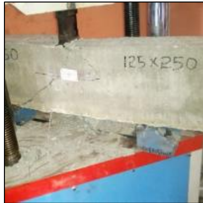
Figure 7 125 x 250 mm Deep Beam after loading to failure
