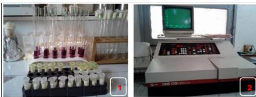
Figure 3 Antioxydant and free radical scavenging assay: colorimetric method with DPPH (1), spectrophotometer analysis (2)
