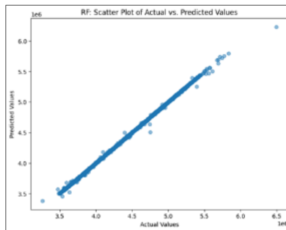
Figure 29 Random Forest Scatter Plot of Actual vs. Predicted Pore Pressure (Test Data)
