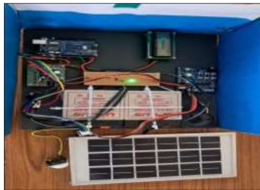
Figure 15 Fabrication of solar bird scarer
