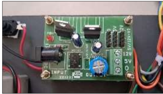
Figure 11 Power supply board
