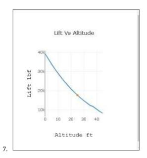
The lift vs altitude graph shows a decreasing non uniform trend. The non-uniform decrease in lift with altitude is primarily due to the reduction in air density and changes in aerodynamic conditions, leading to complex interactions that are not linear across all altitudes.
