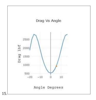
A parabolic graph of drag versus angle of attack indicates that drag increases with AoA, identifies an optimal angle where drag is minimized, and underscores the importance of understanding drag behavior in relation to lift during flight to optimize performance and efficiency.
