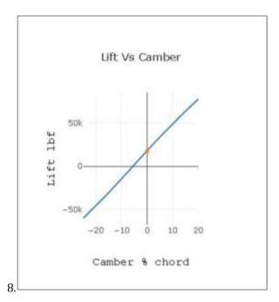
The lift vs camber graph shows that increasing the camber of an airfoil leads to a proportional increase in lift. This indicates that camber is an effective way to enhance lift generation.
