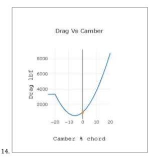
In the drag vs camber graph, the upward slope of the parabola indicates that as camber increases from a low value, drag initially rise. The parabolic relationship highlights the trade-off between lift and drag in airfoil design. While increasing camber can enhance lift, it can also lead to higher drag, necessitating careful optimization for performance.
