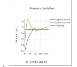
The plot highlights differences in pressure distribution on both surfaces, with a sharp initial peak on the upper surface and a smoother trend on the lower surface. A reference line for the overall pressure is included for comparison.
