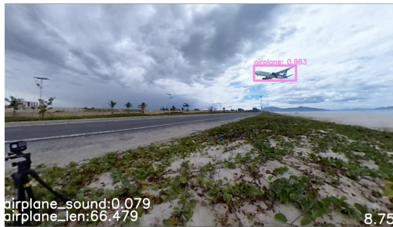
Figure 9 The volume of the sound and the total length of the airplane were shown on the video and visualized
