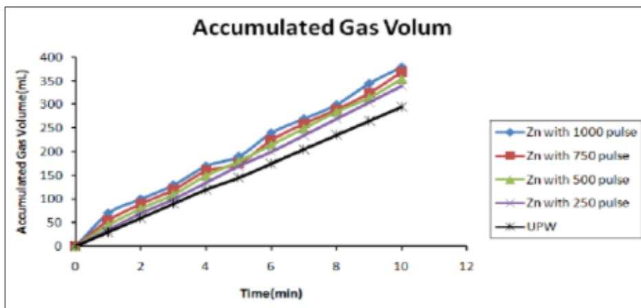
**Figure 2** Accumulated Gas Volume as a Function of Time with Ultrapure Water and with  $\text{Fe}_2\text{O}_3$  and ZnO Nanoparticles Synthesized at different Number of Pulses
