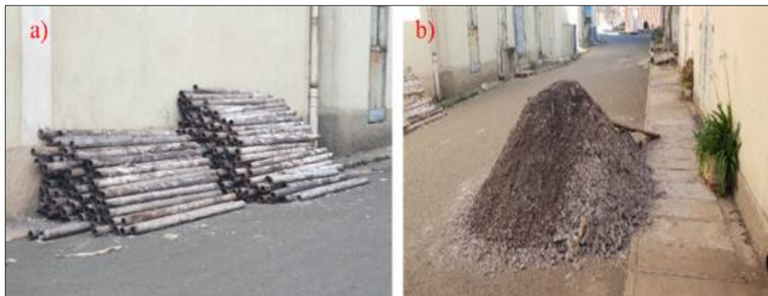
Figure 4 a) Fire tubes with scaling b) Scaling removed from the tubes
