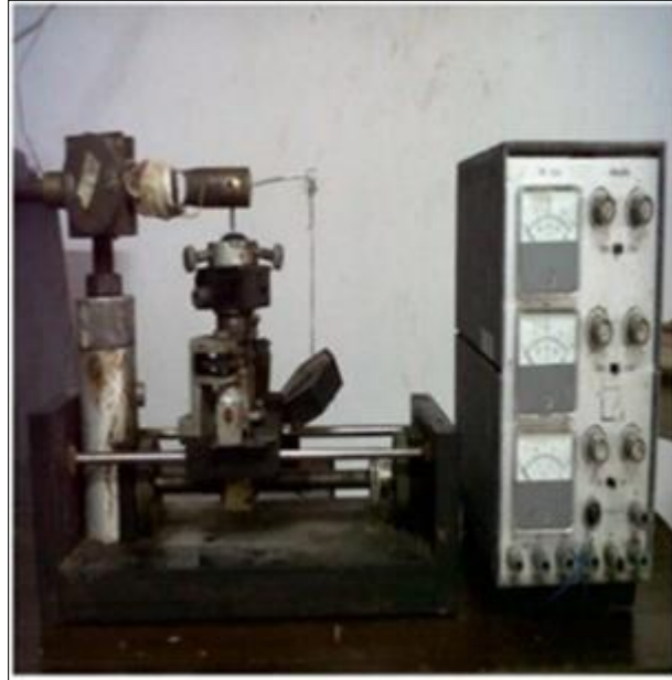
Figure 2 The pin-on disc wear testing
