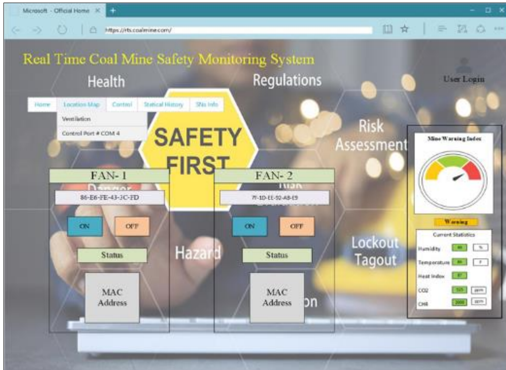
Figure 9 A computer screen view of the interface that was built for turning auxiliary fans on and off
