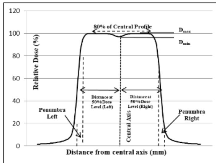
**Figure 1** The measurements of beam profile
