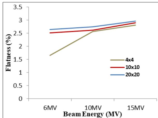
**Figure 13** Variation of flatness with FS for various photon beam at 10 cm depth
