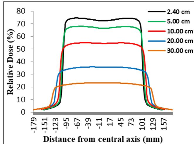
Figure 7 Profile doses curve of 10 MV photon for FS 20x20 cm<sup>2</sup> with various depth
