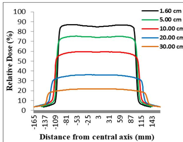
Figure 4 Profile doses curve of 6 MV photon for FS 20x20 cm<sup>2</sup> with various depth
