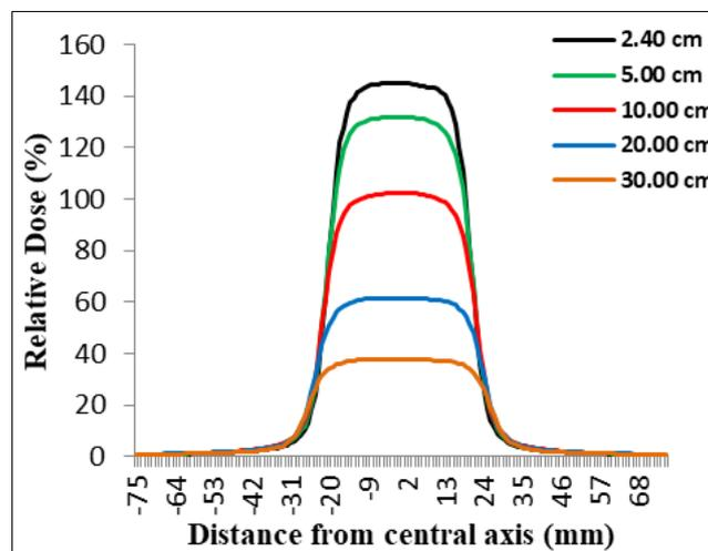
Figure 5 Profile doses curve of 10 MV photon for FS 4x4 cm<sup>2</sup> with various depth
