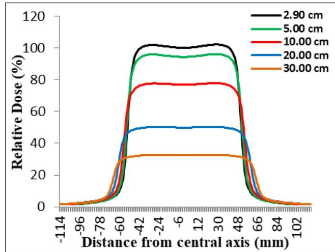
**Figure 9** Profile doses curve of 15 MV photon for FS 10x10 cm<sup>2</sup> with various depth
