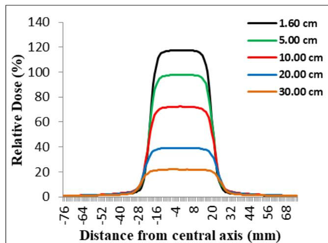
**Figure 2** Profile doses curve of 6 MV photon for FS  $4 \times 4$  cm<sup>2</sup> with various depth
