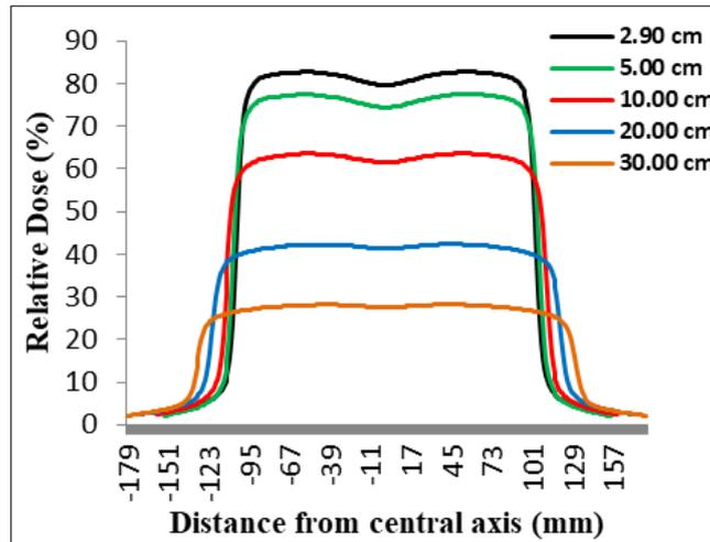
**Figure 10** Profile doses curve of 15 MV photon for FS 20x20 cm<sup>2</sup> with various depth
