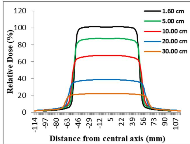
Figure 3 Profile doses curve of 6 MV photon for FS 10x10 cm<sup>2</sup> with various depth
