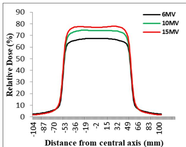
**Figure 11** Profile doses curve of various photon for FS 10x10 cm<sup>2</sup> with 10 cm depth
