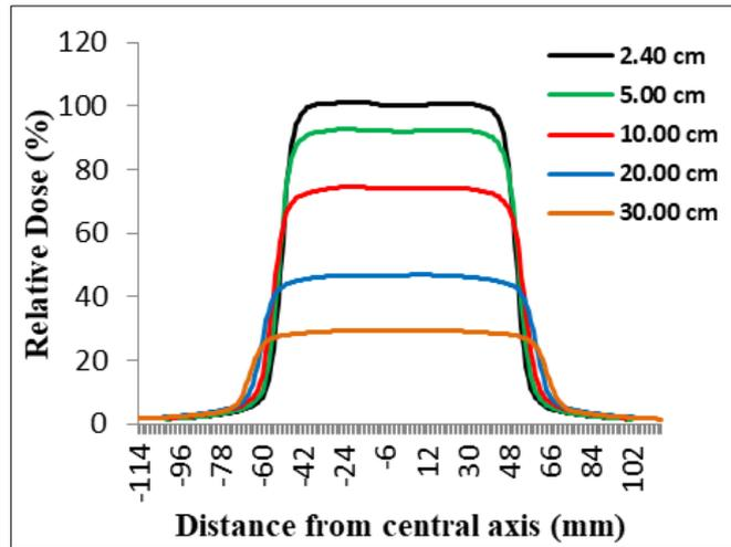
Figure 6 Profile doses curve of 10 MV photon for FS 10x10 cm<sup>2</sup> with various depth
