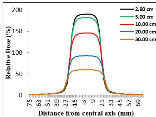
Figure 8 Profile doses curve of 15 MV photon for FS 4x4 cm<sup>2</sup> with various depth
