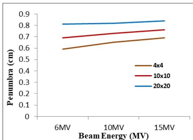
**Figure 15** Variation of penumbra with FS for various photon beams at 10 cm depth
