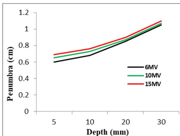
**Figure 14** Variation of penumbra with depth for various photon beams with FS 10x10 cm<sup>2</sup>
