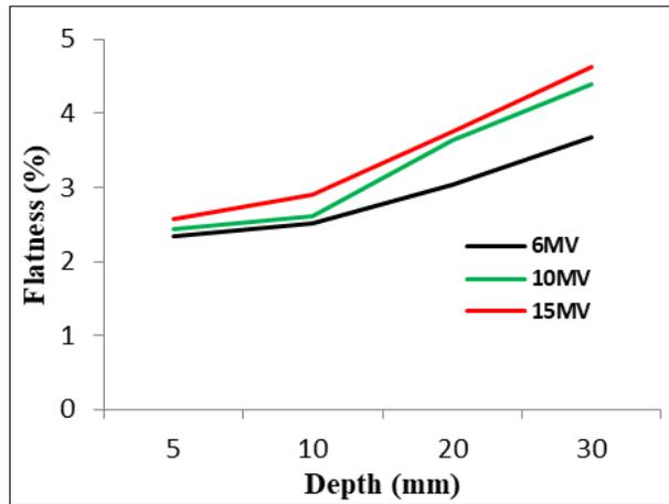
**Figure 12** Variation of flatness with depth for various photon beams with FS 10x10 cm<sup>2</sup>
