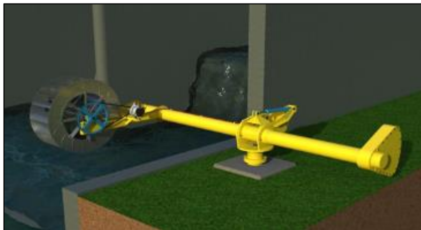
Figure 7 Design Undershoot Waterwheel
