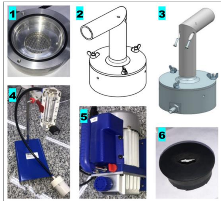
Figure 5 (1) - Capture chamber; (2) - Impactor design of a proposed stage; (3) - Overview of the 3D drawing of the IMPACTOR of a stage; (4) - Flow meter, capacity 50 l/min.; (5) - Vacuum pump, capacity of 60 l/min. and 6 - Nozzle
