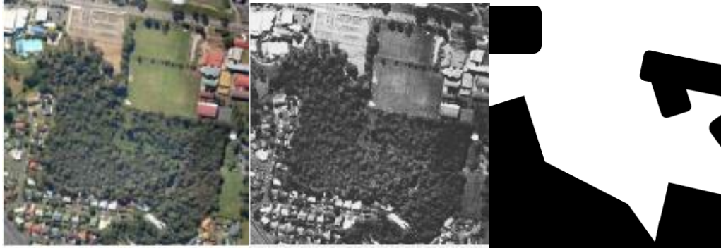
Figure 4 Example for converting the safe zone in white and unsafe zone in black.
