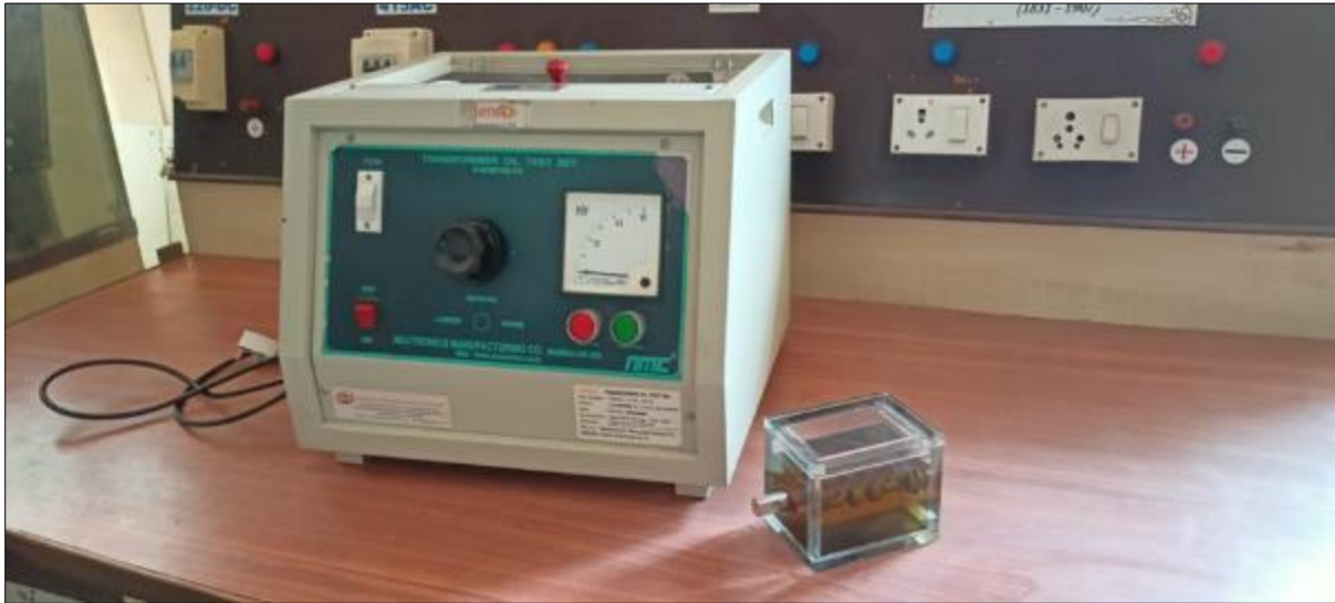
Figure 4 Transformer oil apparatus
