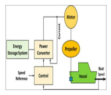
Figure 2 Electric propulsion system components
