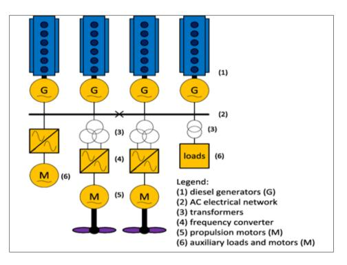
Figure 1 Typical electrical propulsion system layout
