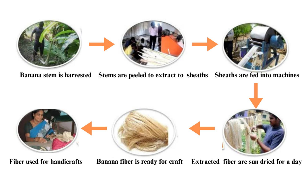
Figure 2 Extraction of fibers from banana stems [adopted from Ortega et al. 2016 [32]]
