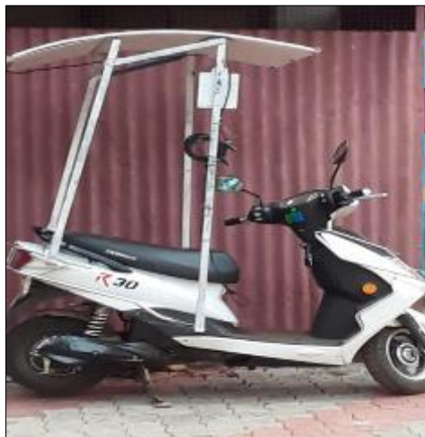
Figure 6 Fabricated Solar panel assisted Electric scooter
