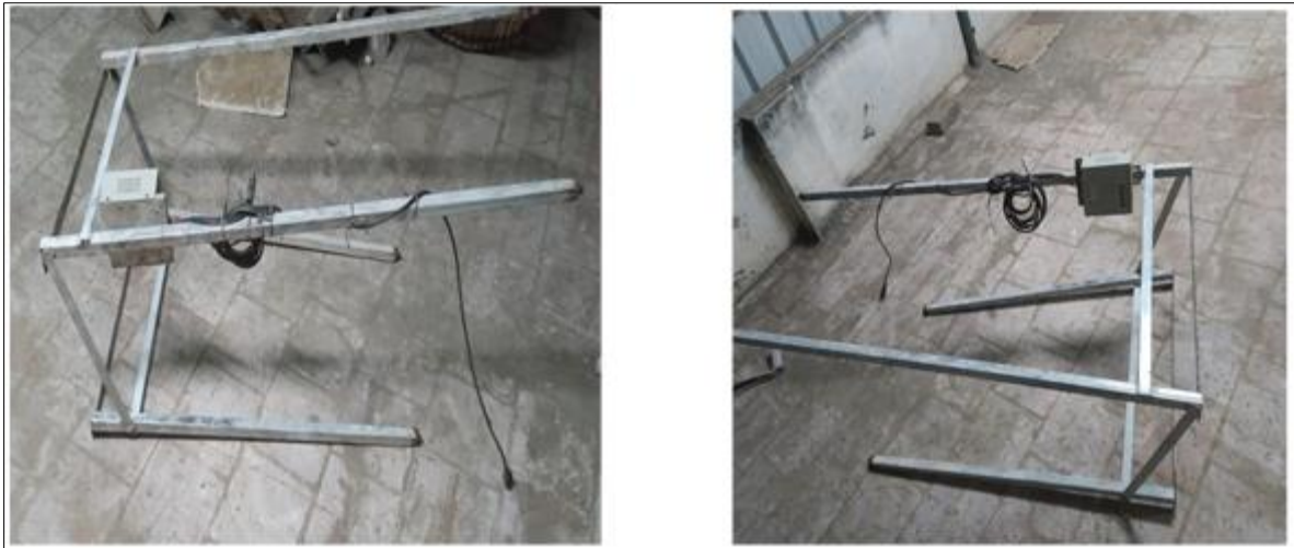
Figure 5 Welded panel stand
