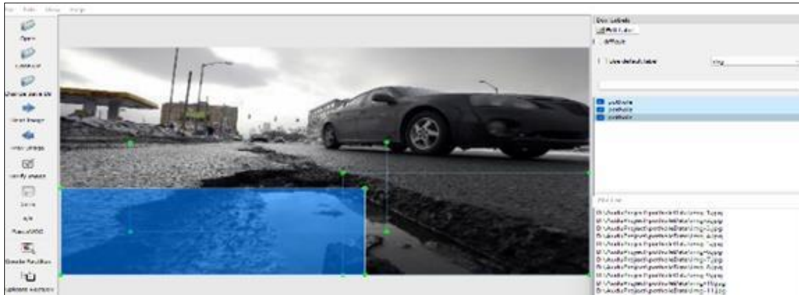
Figure 1b Sample Image Label for Potholes
