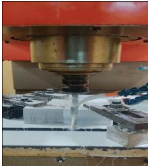
Figure 14 Raw material 70 x70 x 60 mm
