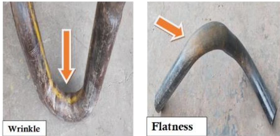
Figure 3 Defects of tube bending
