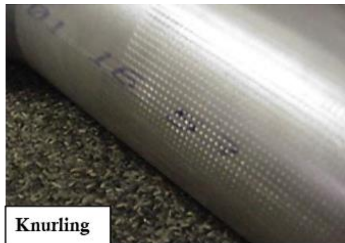
Figure 4 Defects of tube bending
