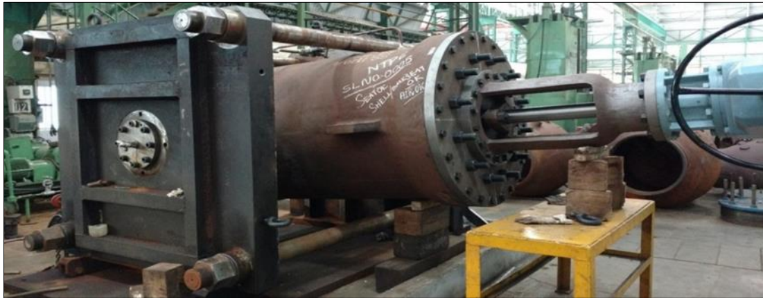
Figure 7 38 - 600 class Gate valve hydro Testing of newly designed and fabricated fixture assembly
