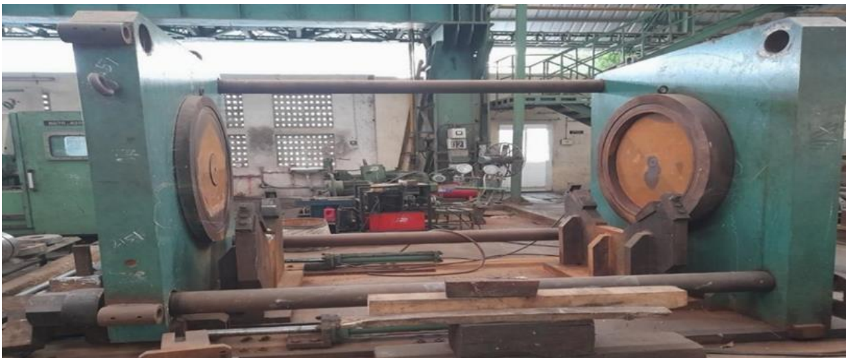
Figure 6 Newly designed and fabricated fixture assembly for big size valve hydro testing
