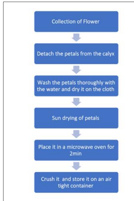
Figure 1 Flowchart of process of drying of blue pea flowers ( Clitoria ternatea )
