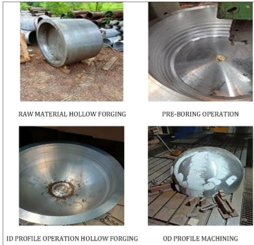
Figure 9 Photos for machining hollow forging
