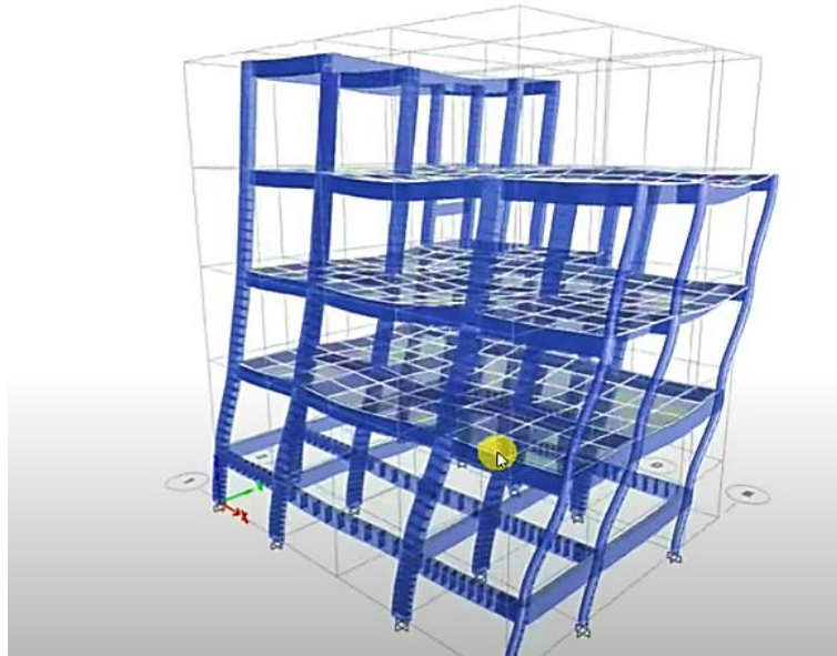
Figure 4 Deflection in the Structure
