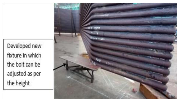
Figure 6 Newly developed lug plate fit up method
