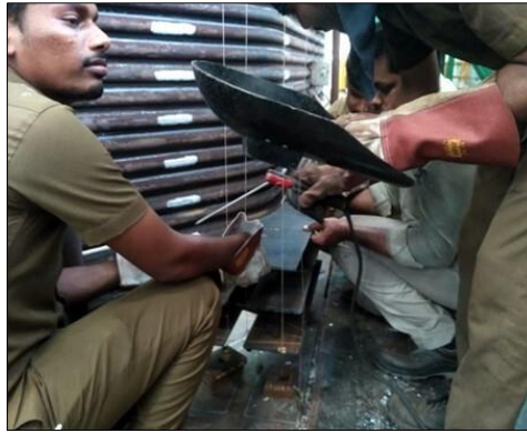
Figure 2 Conventional lug plate fit up method
