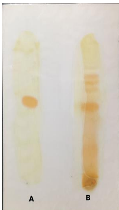
Figure 4 TLC analysis. Lane A -standard vindoline; lane B -ethanolic extract
