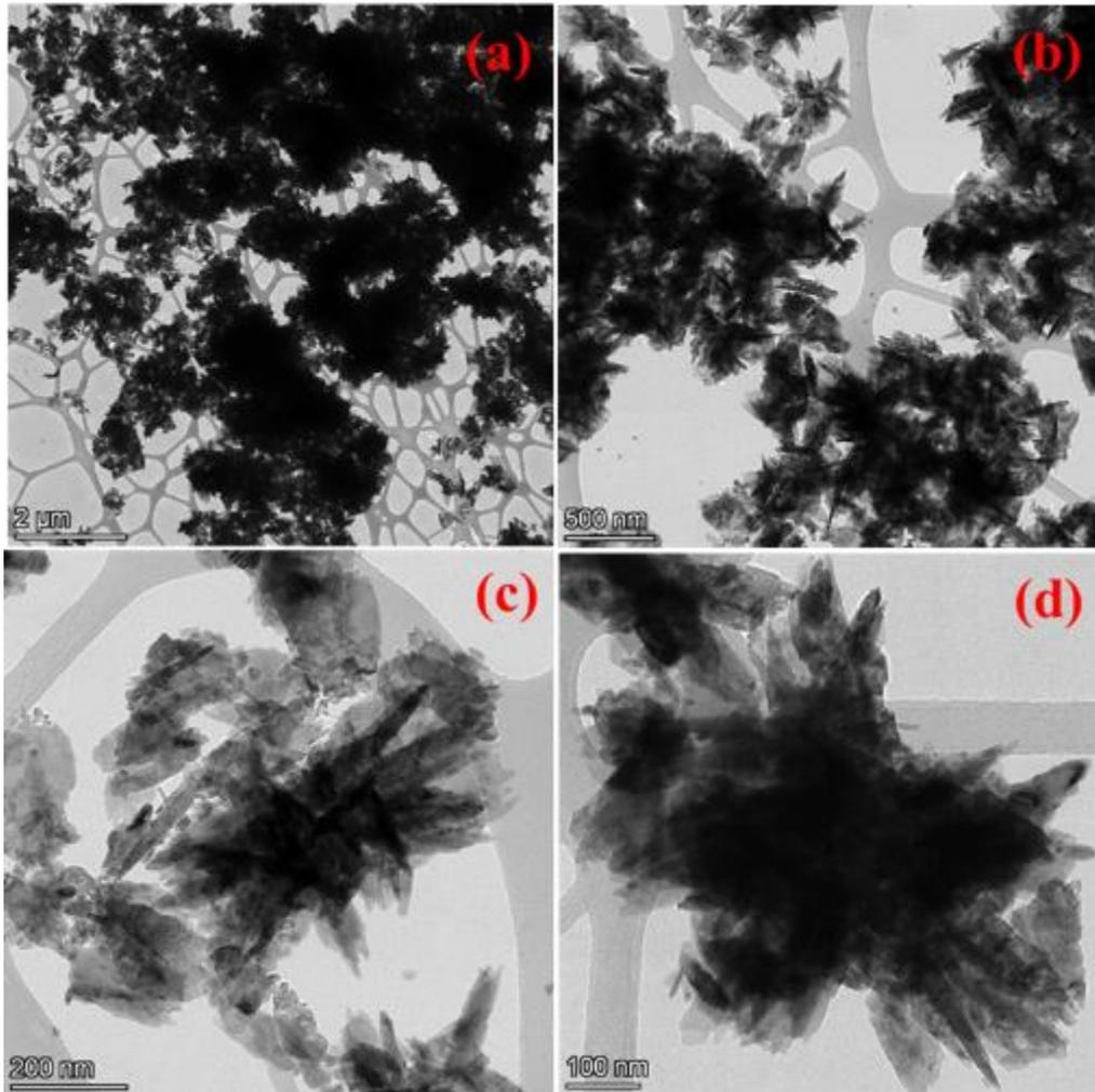
**Figure 5** High Resolution Transmission Electron Microscope (HR-TEM) analysis of synthesized ZONs of *Andrographis alata* ethanol extract: (a)  $2 \mu\text{m}$  (b)  $500 \text{ nm}$  (c)  $200 \text{ nm}$  and (d)  $100 \text{ nm}$
