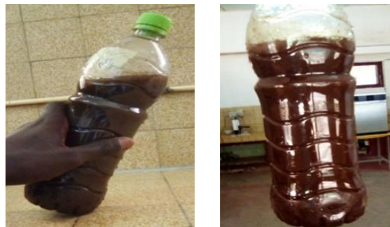
Figure 2 Digestate filtrate to be recycled for biogas production
