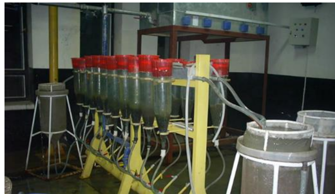
Figure 2 Closed circulatory incubation system for fish eggs incubation (Zoug jar) Switzerland system in Al-Wahda fish hatchery
