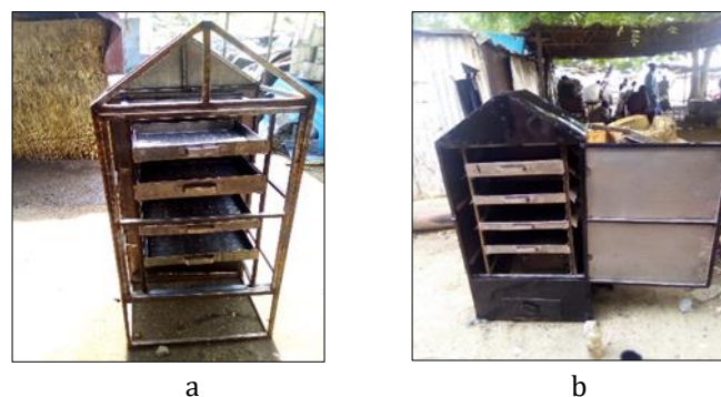
Figure 4 Construction of the cupboard kiln, a) cupboard being assembled b) final cupboard kiln
