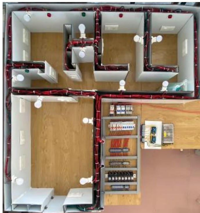
Figure 2 Smart home electrical training model
