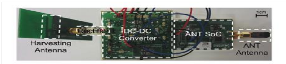
Figure 6 The wearable platform prototype that utilizes readily available components
