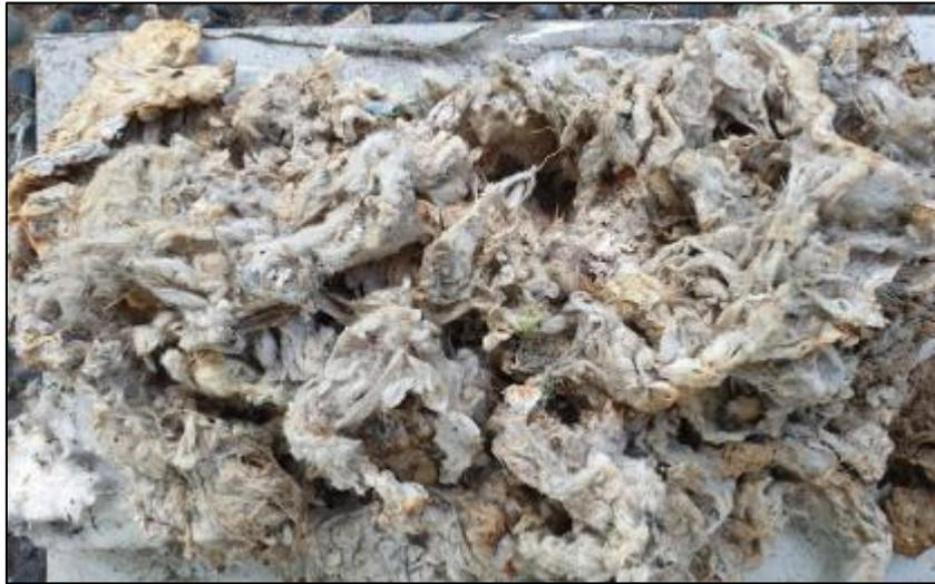
**Figure 3** Cellulose fiber obtained from hydrothermal processing
