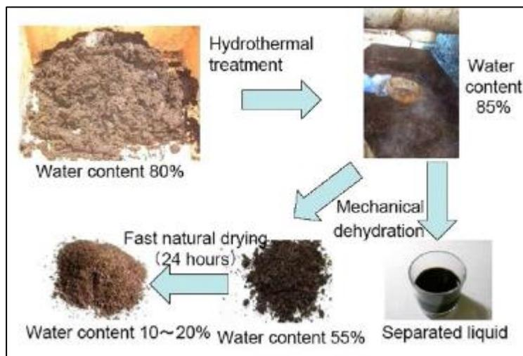
**Figure 2** After the retention time and steam release are completed, the process yields a uniform (homogeneous) sludge product
